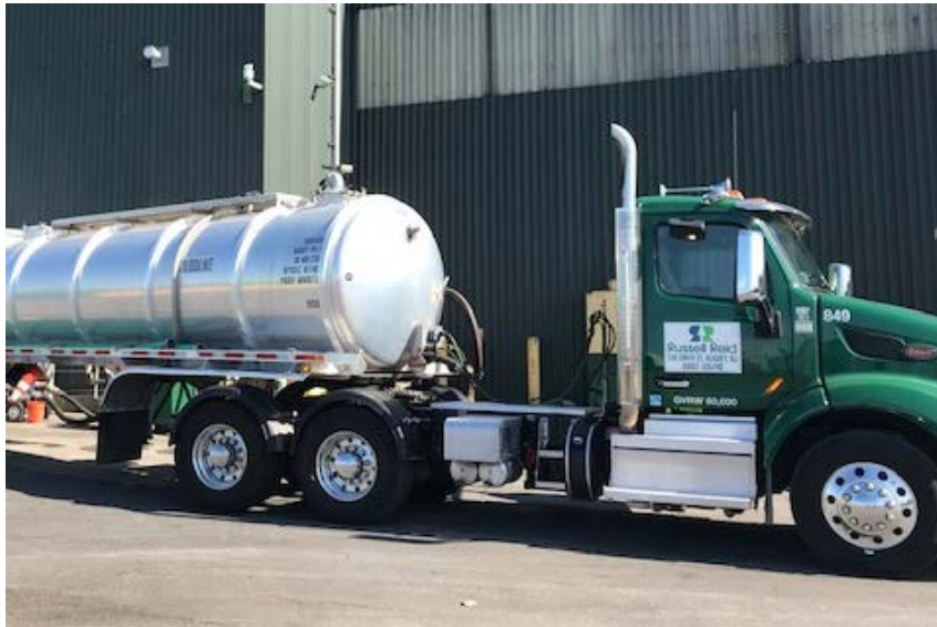
EBS ® is transported to the WWTP via sealed vac truck
